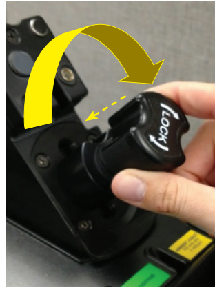
1. Pushing down on the knob, rotate the knob 360 degrees clockwise until it clicks into place.
